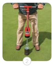
Remove pin. Lift handle and hammer action drives cutter into the ground.
