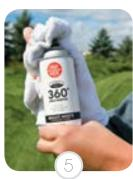
Place rag over nozzle and press to clear excess paint from nozzle after every 9 holes.
